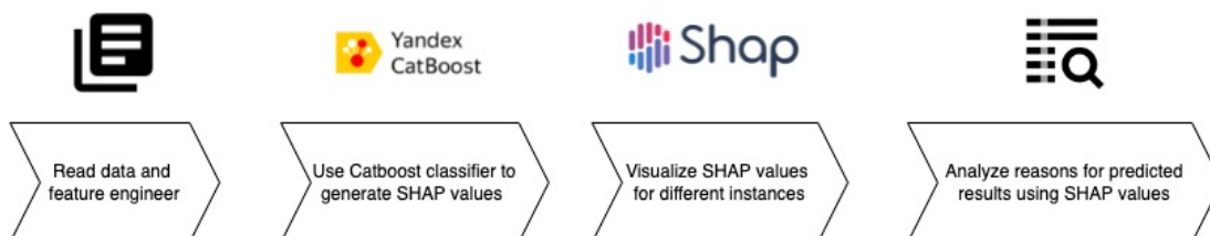
Figure 24: Flow diagram for Explainable AI lab
