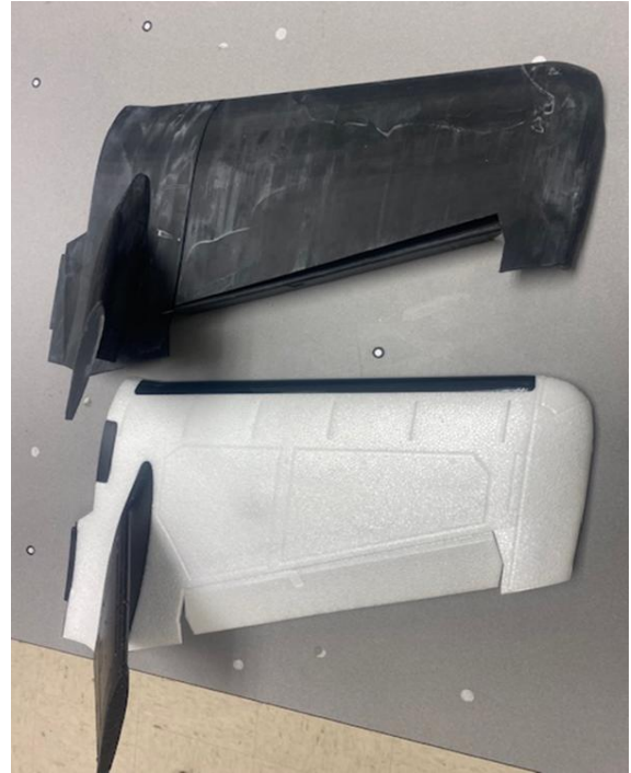
Fig 15: comparison between prototyped part with original one in ZOHD Dart XL drone Finally, all the parts are assembled that are shown in figure 16.
