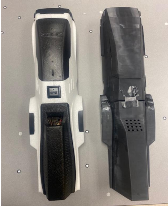
Fig 15: comparison between prototyped part with original one in ZOHD Dart XL drone Finally, all the parts are assembled that are shown in figure 16.
