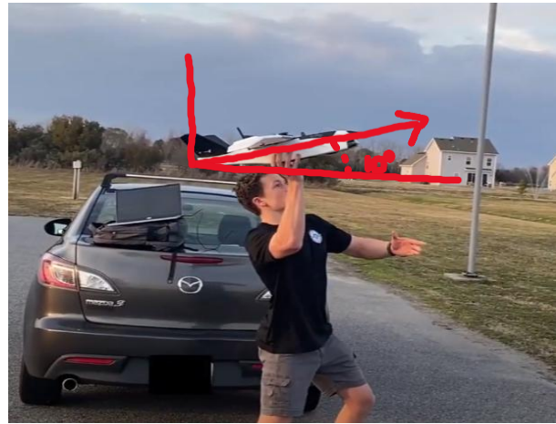
Fig 19: Hand-thrown automatic takeoff
