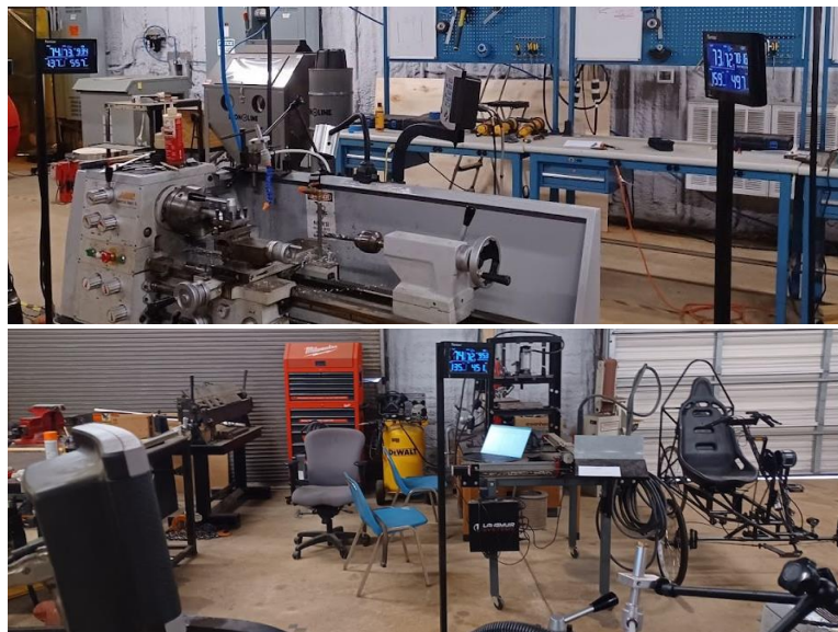
Figure 1: The machining setup with CO 2 sensors in three places around the lathe for the experimentation
