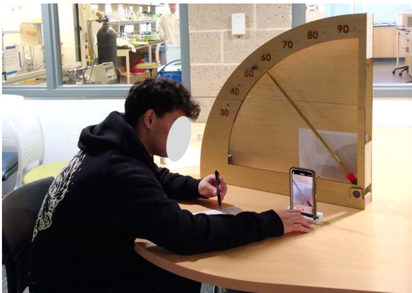
Fig. 9. A student video recording the collar-spring impact
