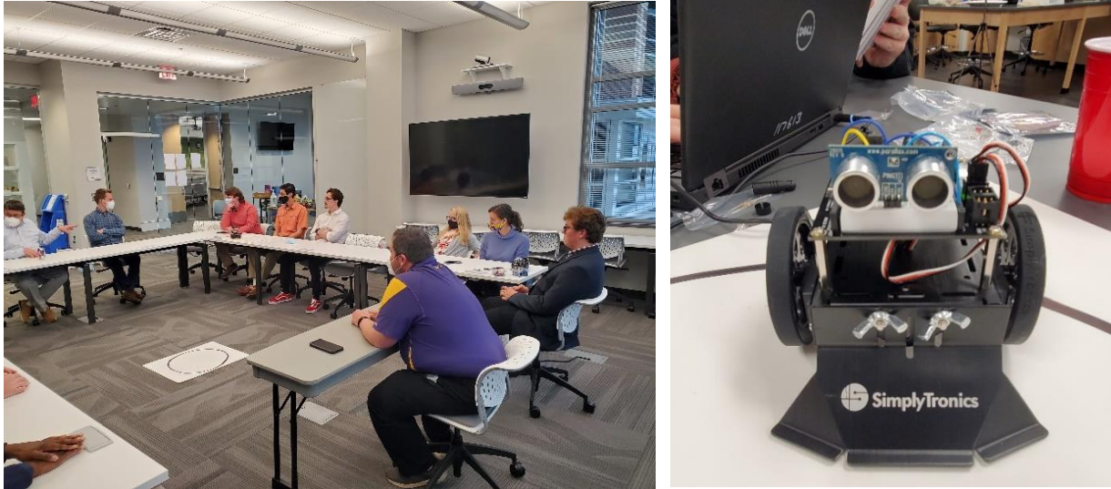
Figure 2 Left) Students and Faculty prepare for the Sumo Robot Competition, Right) One of the sumo robots with an ultrasonic sensor mounted on top to find an opponent and a bumper to push the opponent out of the ring.
