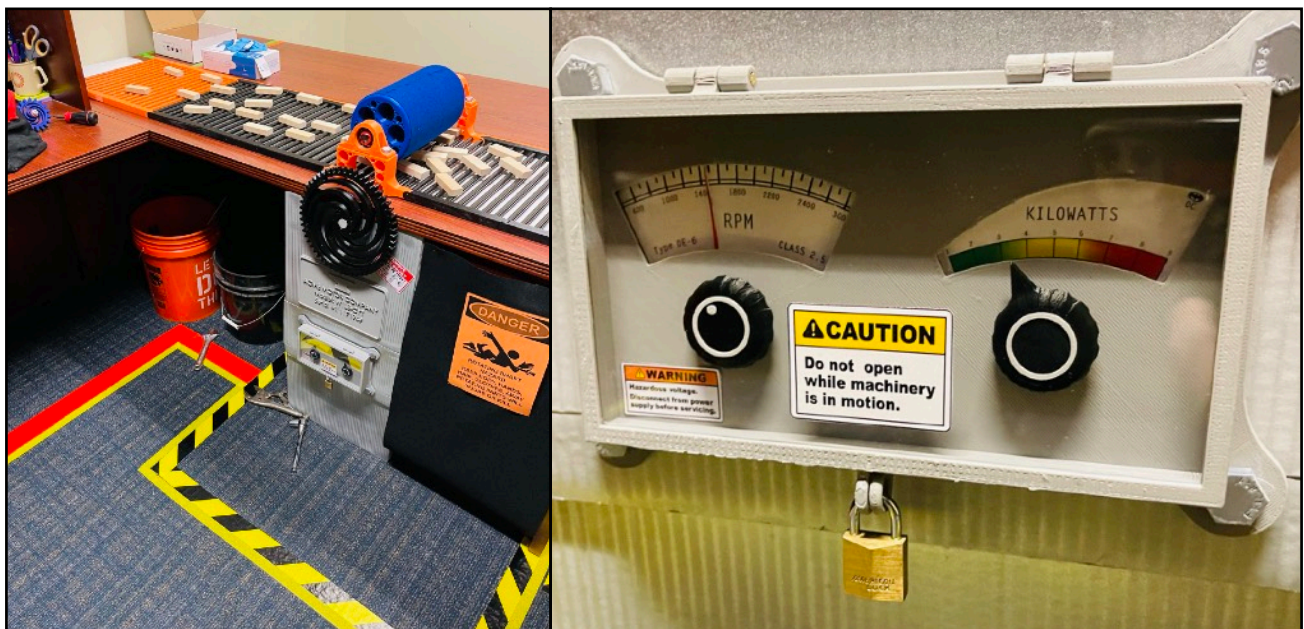
Figure 6: Motor station, and a close-up view of the speed and power indicator.
