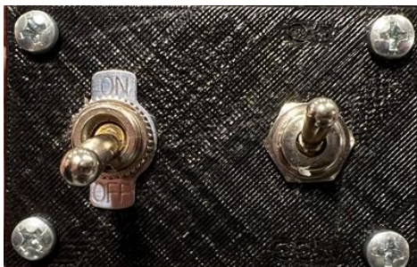
Figure 7. Switchbox to control power and rotational direction of propeller.
