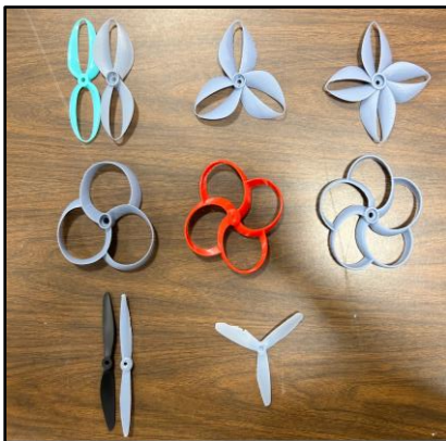
Figure 1. Top row (left to right): Dalprop Donut injection molded toroidal propeller, 2-blade “sharp” printed toroidal propeller, 3-blade “sharp” printed toroidal propeller, 4-blade “sharp” printed toroidal propeller. Middle row (left to right): 3-blade “rounded” printed toroidal propeller, 4-blade “rounded” printed toroidal propeller, 5-blade “rounded” printed toroidal propeller. Bottom row (left to right): 2-blade injection molded standard propeller, 2-blade printed standard propeller, 3-blade printed standard propeller.
