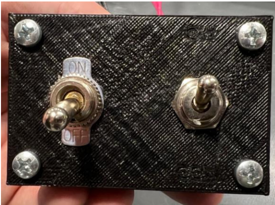
Figure 12. Battery power switch (left) and blade rotation switch (right).
