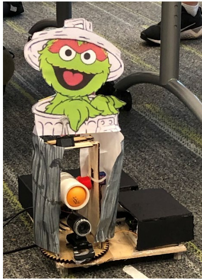
Figure 1: Example ping-pong ball launcher showing the webcam for finding the target so the launcher could be aimed.
