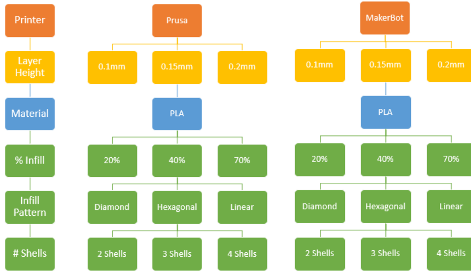
Figure 2 specimen printing and coding configuration
