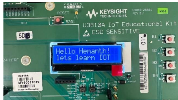
Figure 3. Program output on LCD display.
