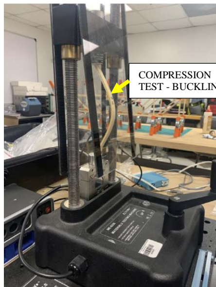
Figure 7: Compression test of bamboo sticks and curve load versus slenderness.
