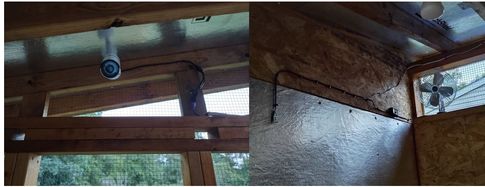
Figure 5. Coop Camera, Fan, light, and DHT sensor
