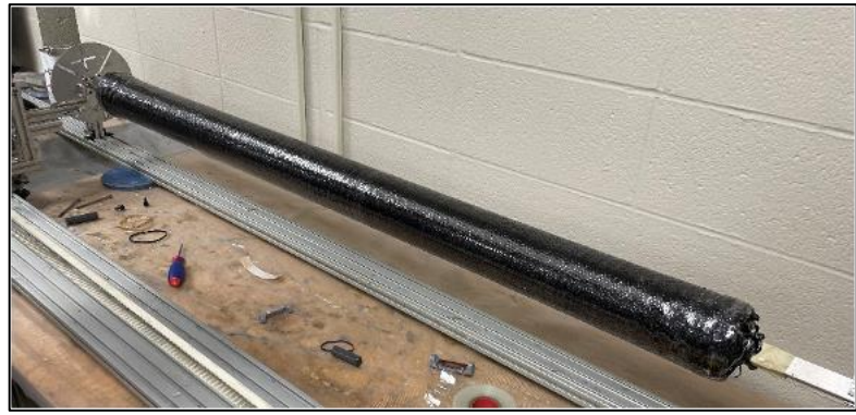
Figure 7: X-Winder Lower Airframe Tube Winding
