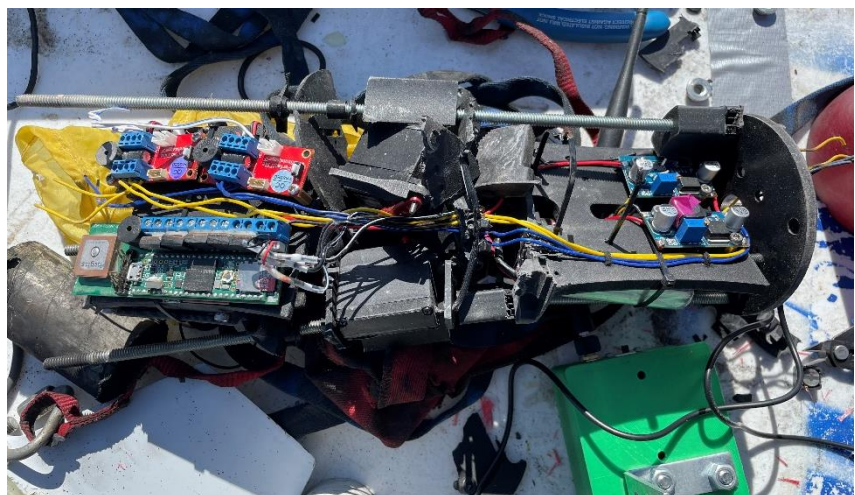
Figure 14: Avionics Bay Damage
