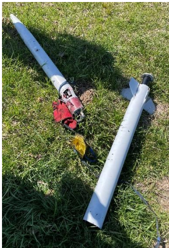
Figure 13: Upper (left) & Lower (right) airframe damage
