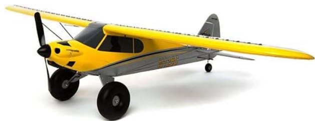
Figure 4. Airplane drone (HobbyZone Carbon Cub S 2).
