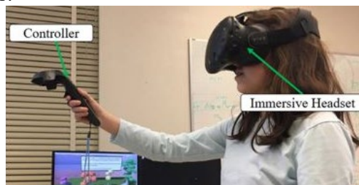
Fig 1: An immersive VR based VLE (the student is wearing a 3D headset and interacting with the target environment using a controller)
