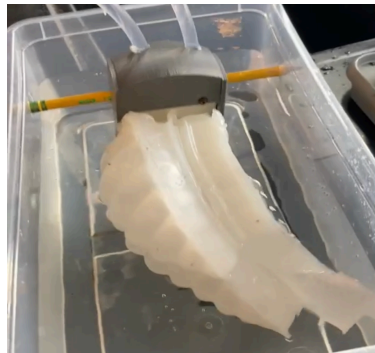
Figure 5: The final prototype demonstrating stationary movement using water pumped from syringes and plastic tubes.
