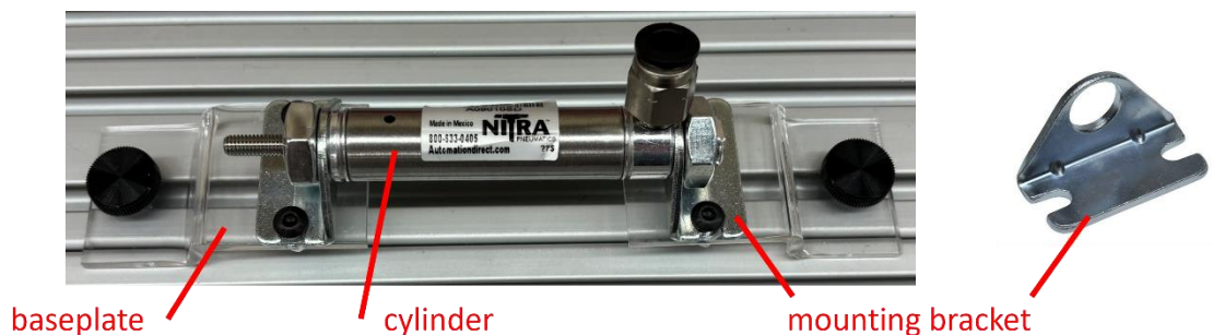
Figure 6: Cylinder mounted to an acrylic baseplate with mount, thumbscrews, and drop-in t-nuts.
