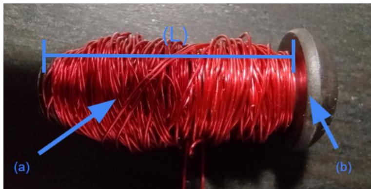
Figure 6: An example of an electromagnet with (a) a hand-wound coil and (b) a magnetic core of a length (L).
