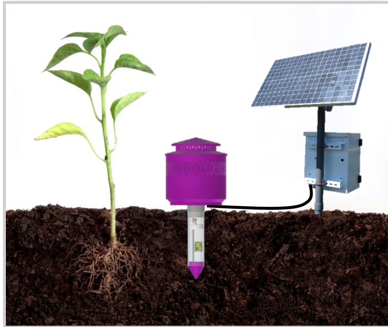
Figure 4. Setup of the minirhizotron in the field.
