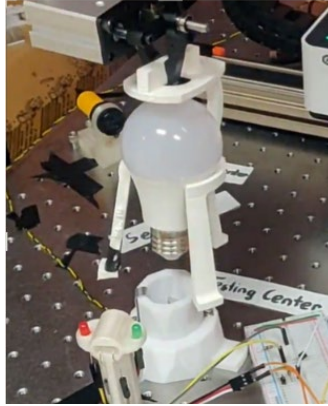
Figure 3. 3D printed bulb holder and testing center.
