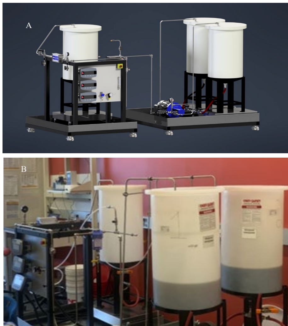
Figure 3: Finalized Pilot Plant: CAD Diagram (A) and Installed Pilot Plant at the Laboratory (B)
