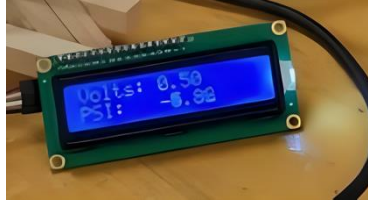
Figure 5. Voltage (Volts) and pressure (PSI) displayed on the LCD
