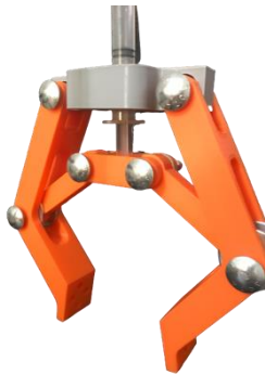
Figure 1. Final assembly of the pneumatic gripper
