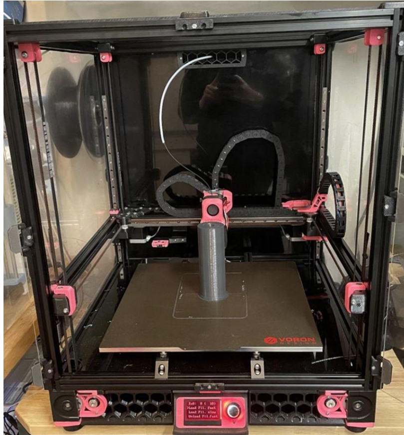
Figure 6 – ABS Fuel Grain Fabrication (3-D Printing)
