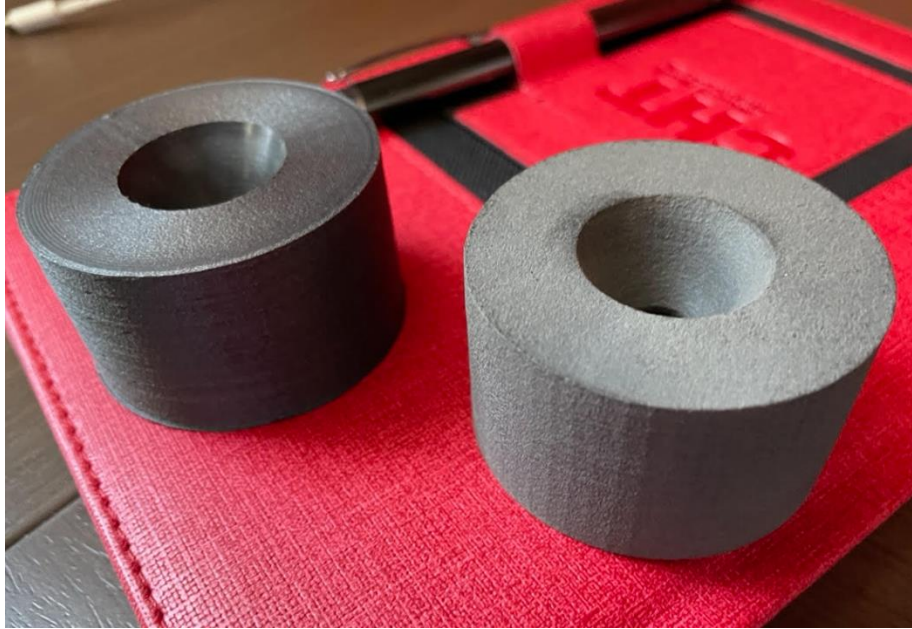
Figure 7 – Graphite (Left) and CBAM (Right) Exhaust Nozzle Test Articles
