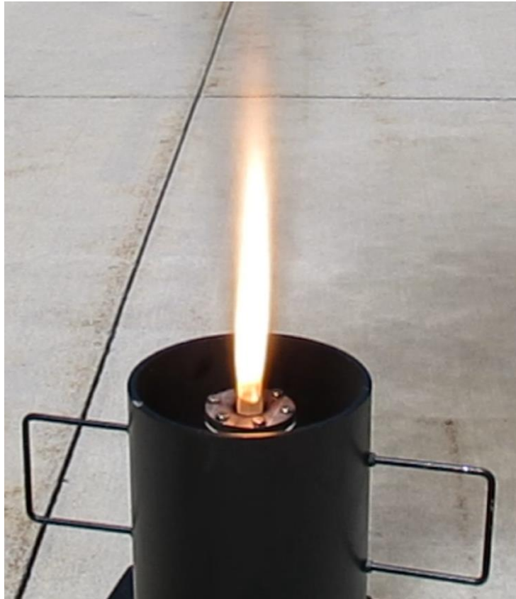
Figure 5 – Concept Hybrid Rocket Demonstrator Exhaust Plume During a Test Firing
