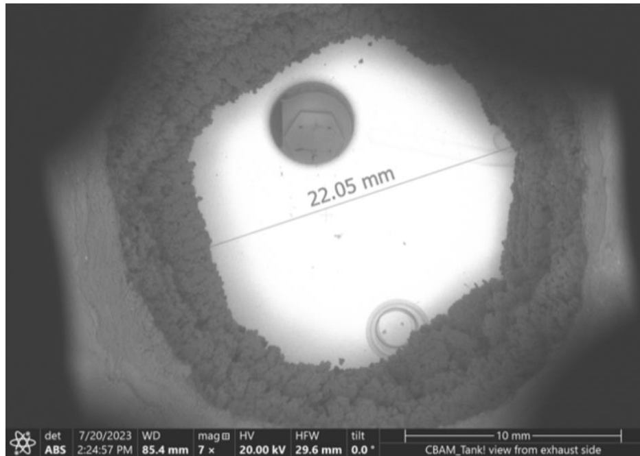
Figure 16 - Post Test CBAM Nozzle Throat (SEM Image)
