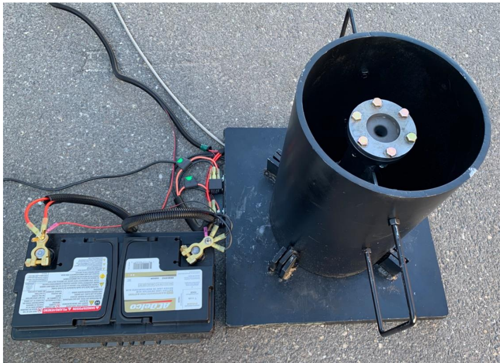
Figure 4 – Pre-Test Rocket Assembly (Containment Shield Installed)
