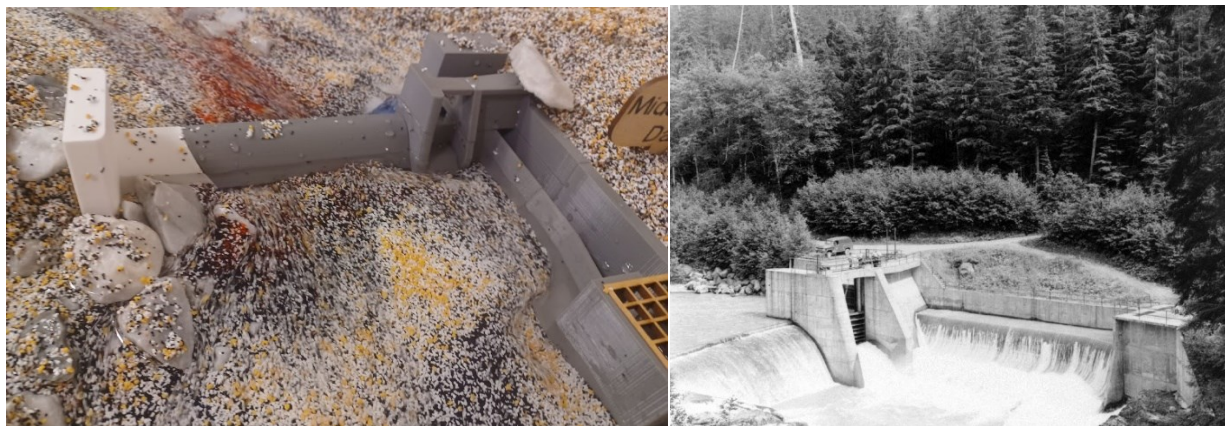
Figure 2. (Left) Student-designed model of a dam used to explore the impact on sediment from dam removal. (Right) Historical photo of the dam (photo credit: Jack Garver).
