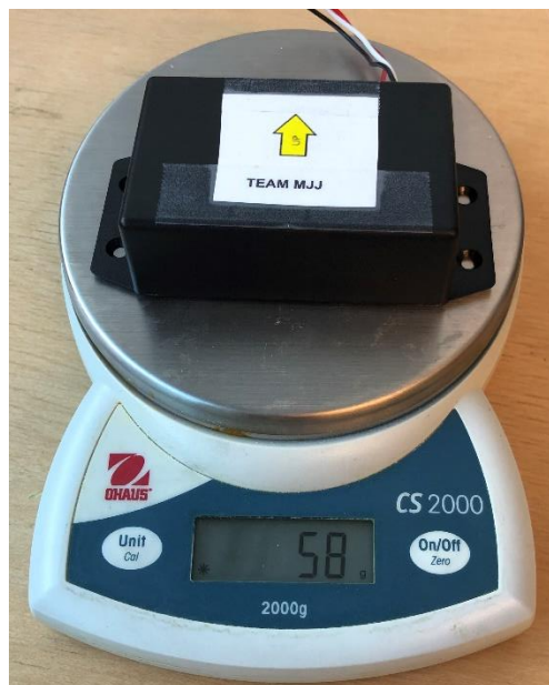
Figure 11. Prototype tilt sensor being weighed.
