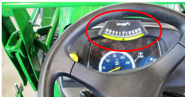
Figure 1. A passive inclinometer installed on a garden tractor.
