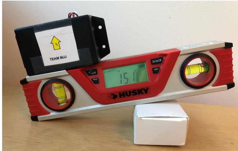
Figure 6. Static testing of tilt sensor using a digital level as tilt angle reference
