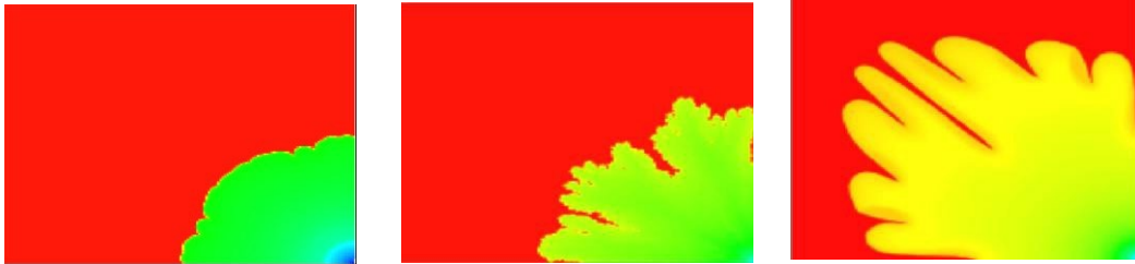
Fig. 7-Schematic showing simulated viscous fingering in water, oil, and mixed wet in a homogeneous rock system.
