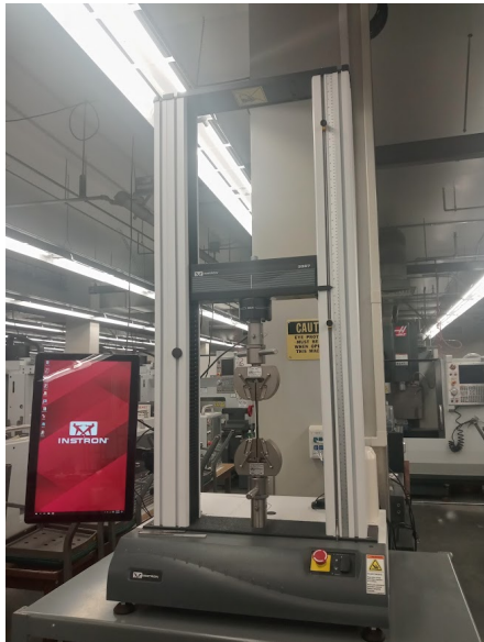
Fig 7. Dogbone specimen set up in the Universal Testing system for a tensile strength test.
