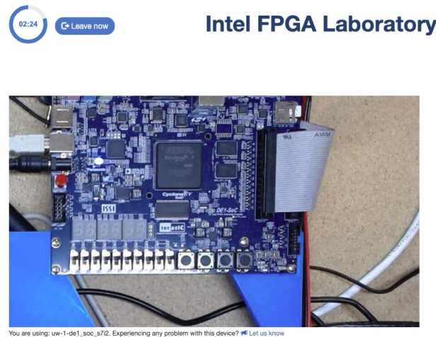
(c) Student's view of the remote FPGA boards via a webcam.
