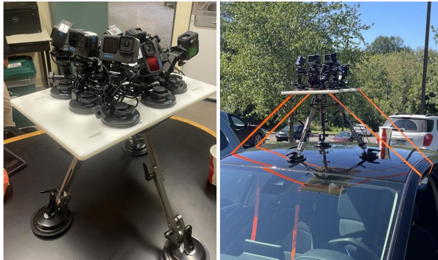
Figure 2. (a) Set of seven cameras (five GoPro and two Mapir cameras). (b) Set of cameras assembled on top of a vehicle for data collection.
