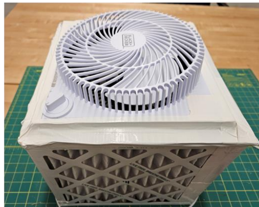
Completed C-R Box!
