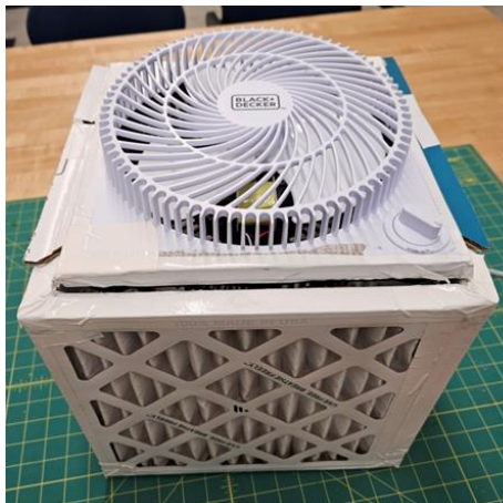
Place the fan on the filter box and tape all edges firm with DUCT TAPE!
