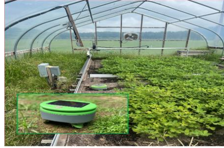
Figure 1b. View from inside of outdoor Farmbot with solar-powered robotic weeder
