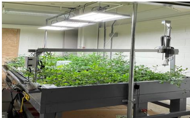
Figure 2. Indoor FarmBot with Growlights, the Farmbot bed is on a mobile table
