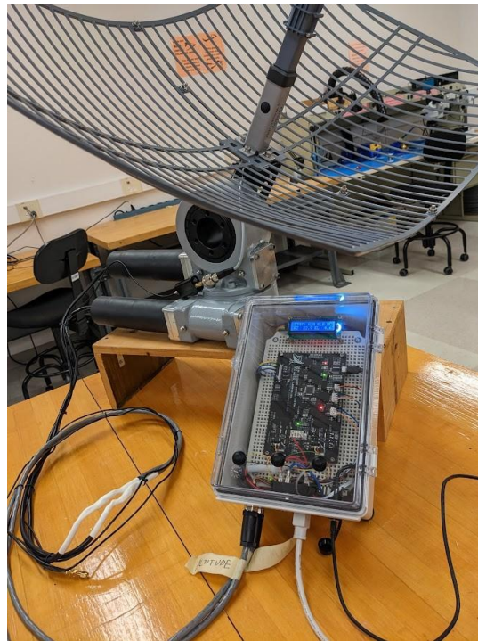
Figure 9: Final Configuration of Prototype, Using 1-Meter Grid Dish Antenna for Testing.
