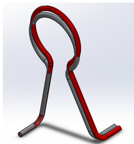
Figure 3, Reference Hook (Red) and Student Hook (Silver) in Assembly to See Differences.
