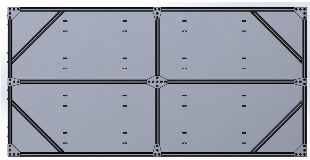
Figure 4: Framing of one module, including external and internal fasteners.
