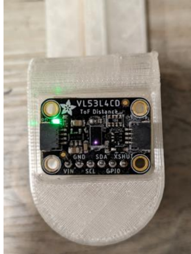
Figure 8. The installed ToF sensor.
