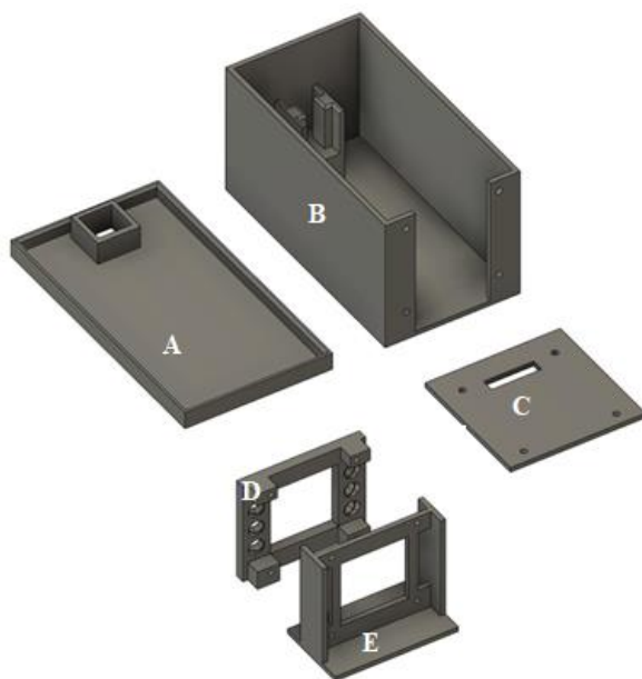
Figure 1. The cover of the spectrometer (A). The base of the spectrometer box with an integrated semi-micro cuvette holder (B). The back wall of the spectrometer with a slit to accommodate Raspberry Pi Camera ribbon cable and wires for LED power (C). The bracket is to hold six white LEDs (D). The mounting bracket for the Pi Camera (E).
