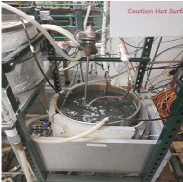
Figure 4. “Large tank” (coil heat exchanger) temperature setup: picture and basic diagram
