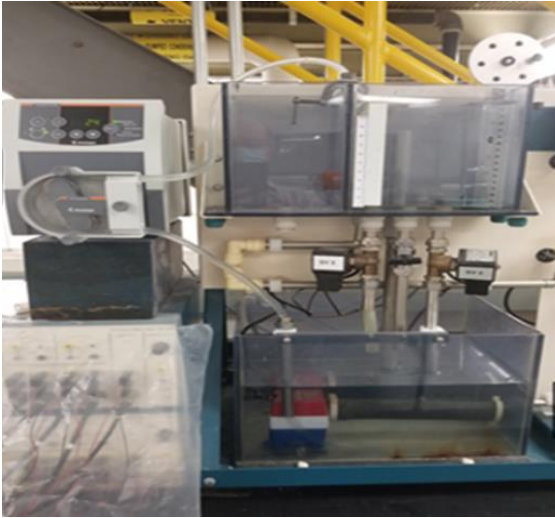
Figure 1. “Small tank” liquid level setup: picture and basic diagram
