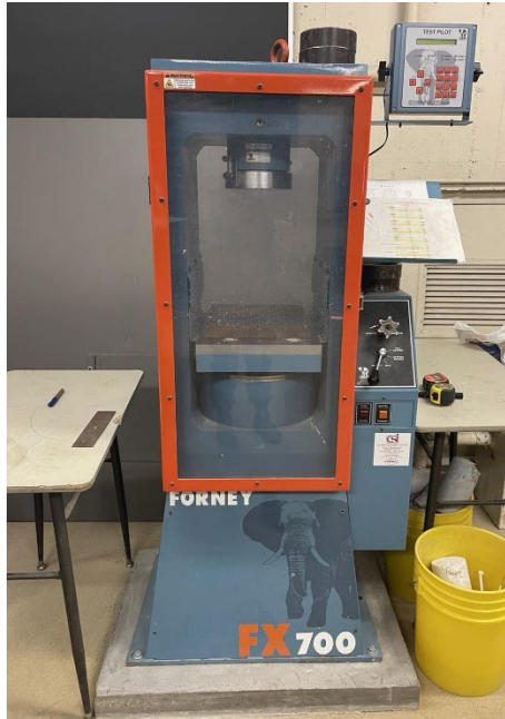
Figure 6. (a) Forney Compression and Tension machine (b) 4-point bending test of small reinforced concrete beam
