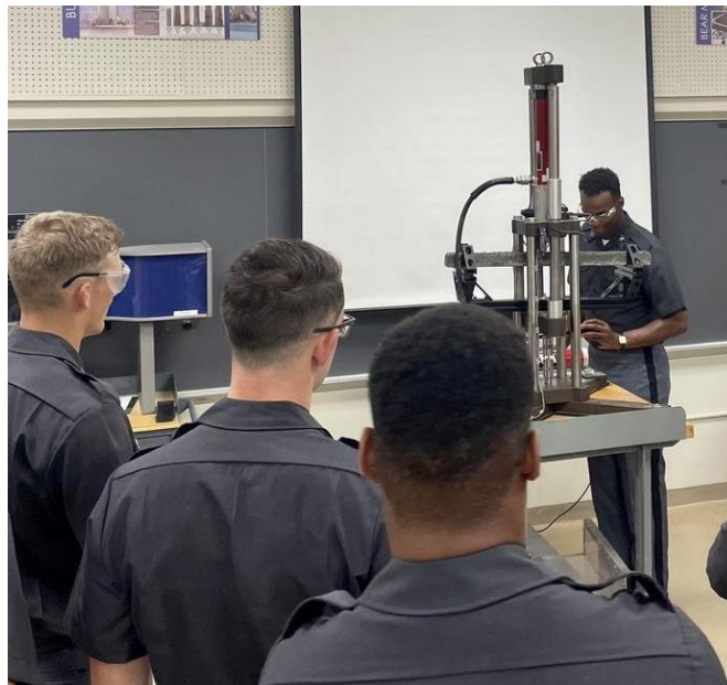
Figure 4. Reinforced Concrete Beam Demonstration with UTM
