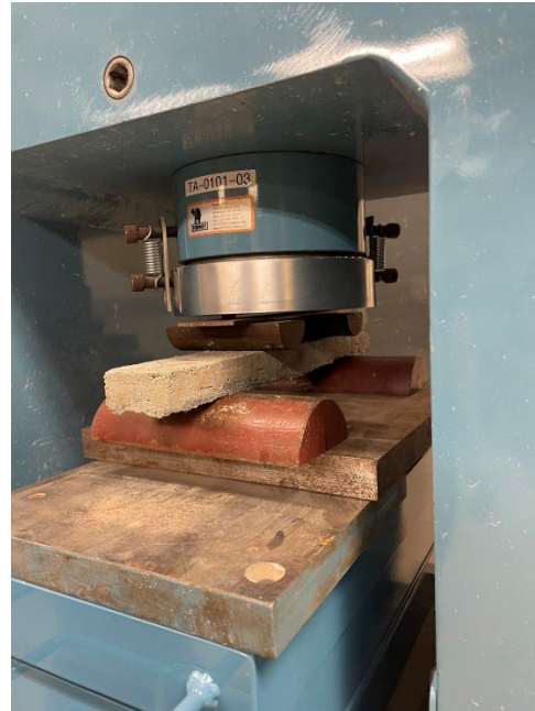
Figure 6. (a) Forney Compression and Tension machine (b) 4-point bending test of small reinforced concrete beam
