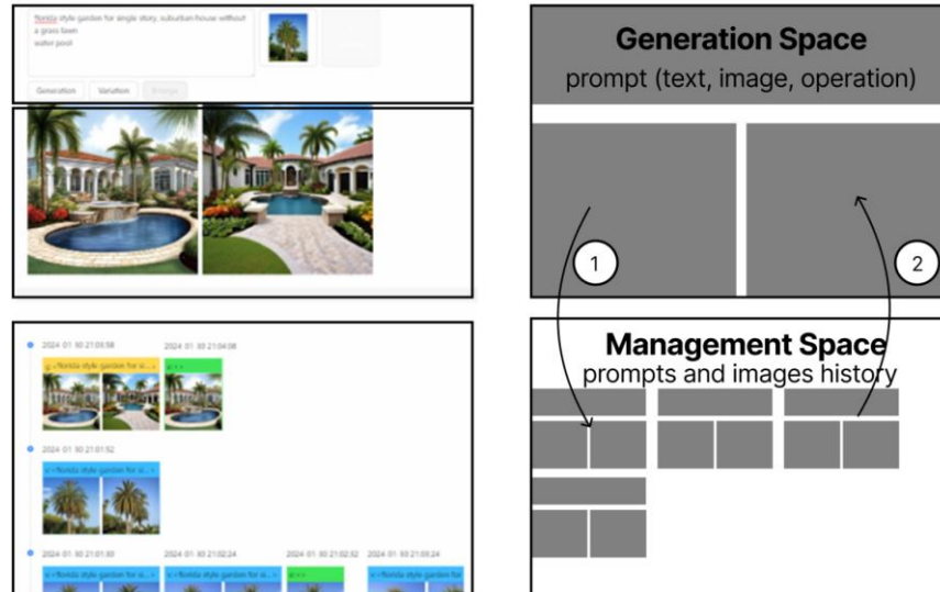
Figure 3. An interface design of how management space interacts with generation space to better enhance design creativity.
