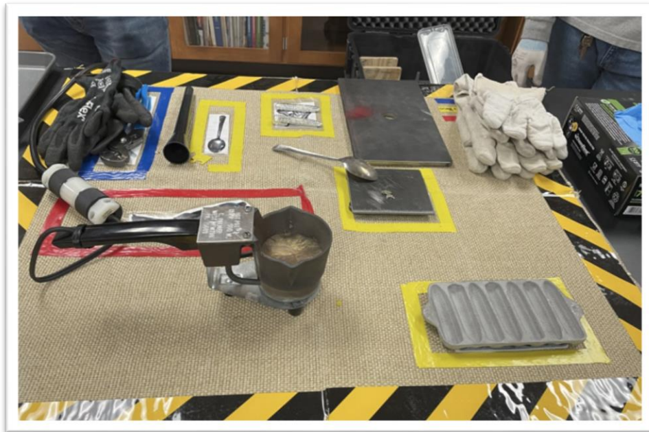
Figure 6. Demonstration set for tin sand casting-prepared by yyyyyy casting plant
