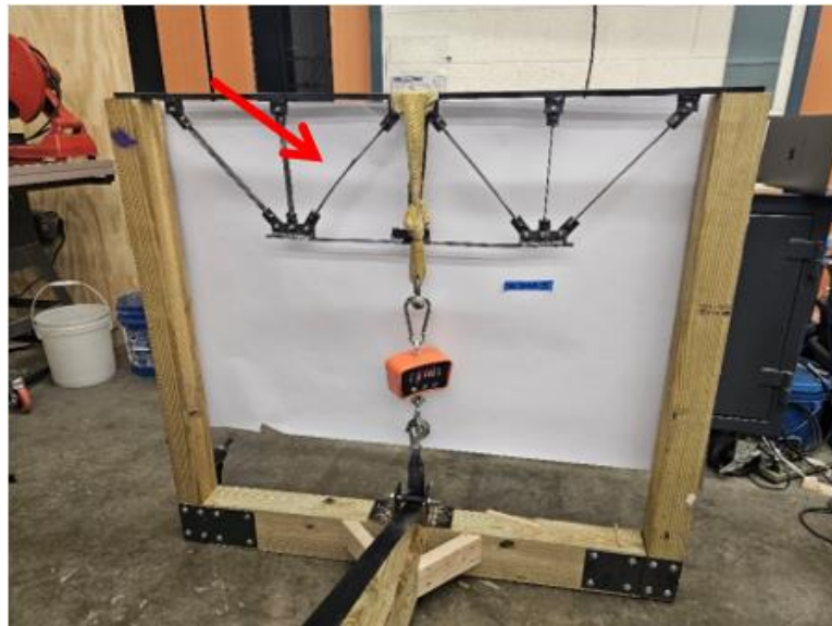
Figure 6: Test setup to mimic designed prototype: Elements show initial buckling failure.
