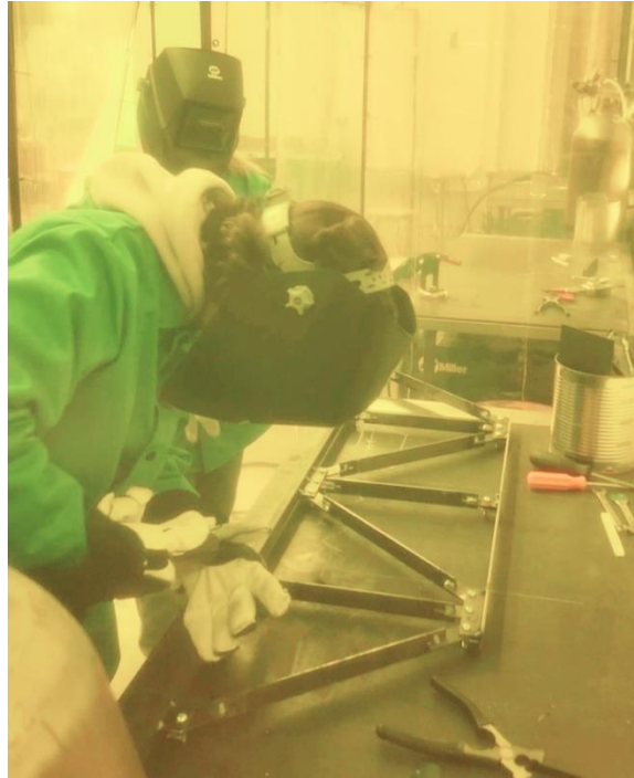
Figure 4: Student welding the prototype truss connections behind a protective screen.
