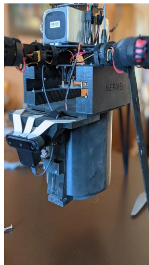
Fig. 8. Fire Suppressant System Design
