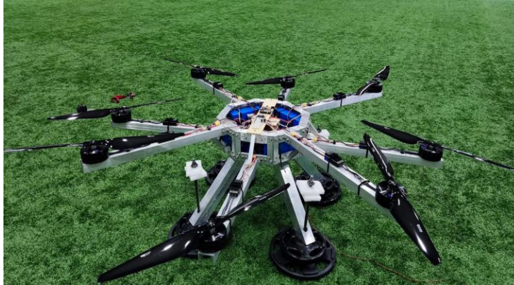
Fig. 5. Octocopter with overlapping propellers
