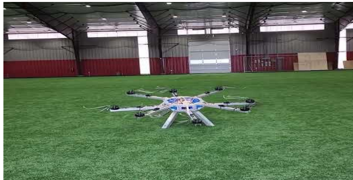
Fig. 6. Octocopter tilting during takeoff indoors
