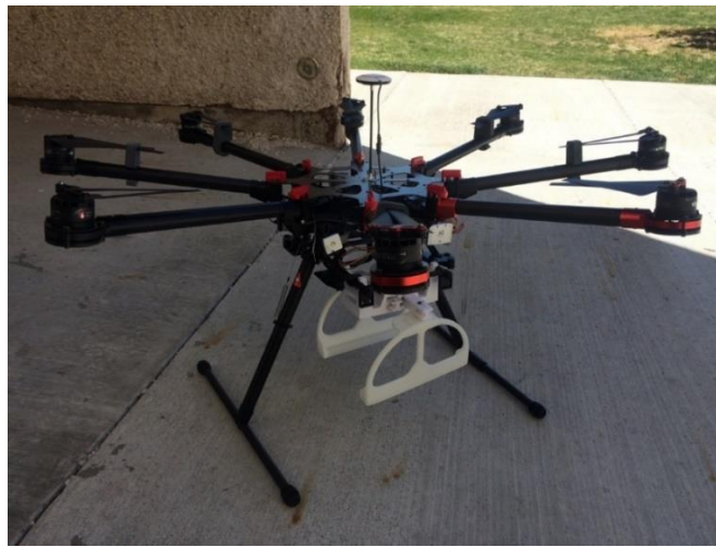
Fig. 2. RTF octocopter designed for package delivery
