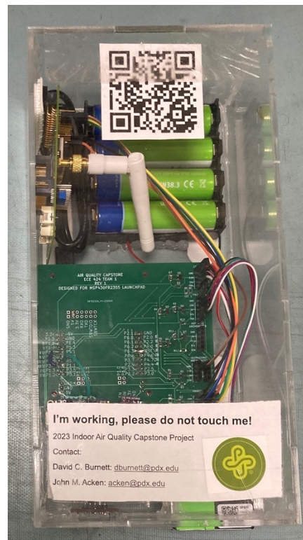
Fig. 3: Year 3 sensor electronics enclosed by custom laser-cut acrylic case with helpful labels attached. Components include 4x 18650 Li-ion batteries, SmartMesh IP development board (vertically-oriented with white antenna protruding in upper left corner), TI MSP430FR5994 development board (under green PCB), custom junction PCB to connect components (green PCB), Sensirion SCD41 carbon dioxide sensor (obscured by white label at bottom) and Sensirion SPS30-PM2.5 particle counter sensor (green sensor protruding from acrylic case along bottom right corner). Project is described in more detail in [4].
