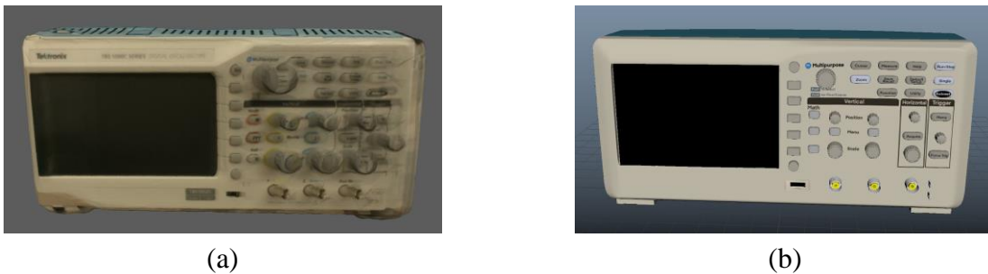
Figure 4. 3D models of an oscilloscope. (a) The original 3D model is directly generated by the 3D scanner. (b) The final 3D model that was generated using Maya based on the original model.
