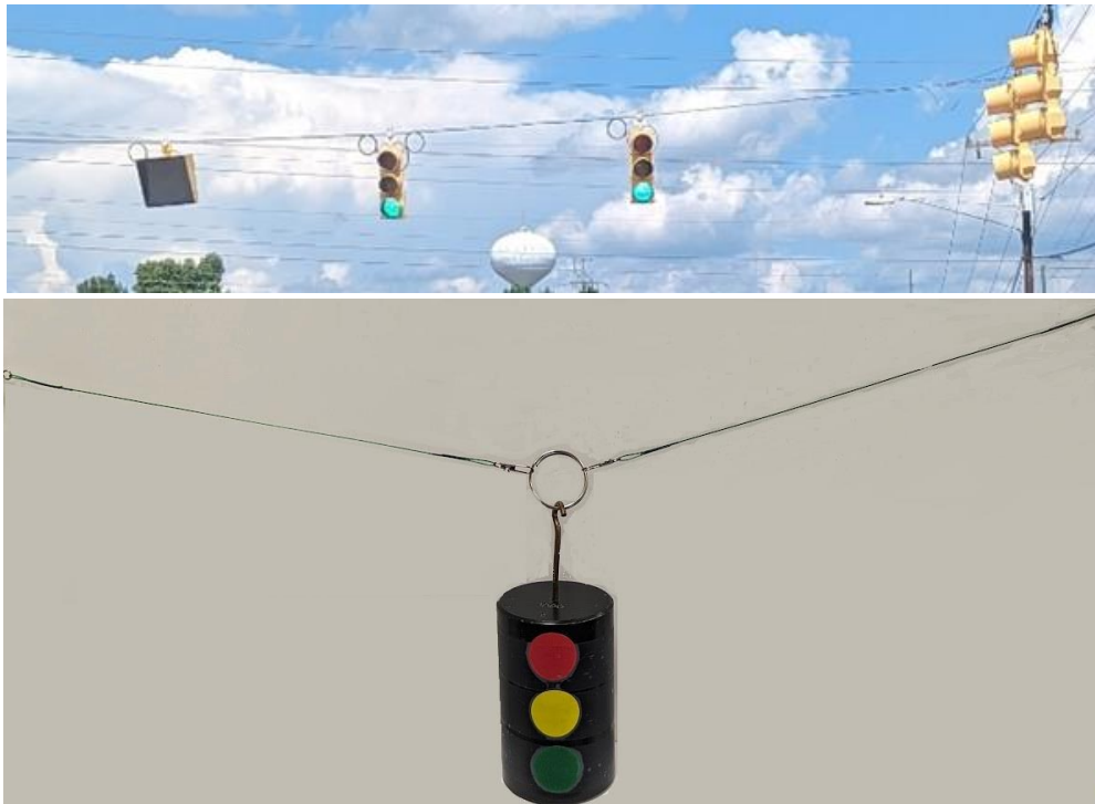
Figure 2. Images of cable-supported traffic lights (top) and an analogous model of a weight supported by cables (bottom).
