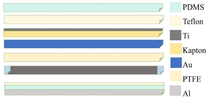
Figure 6 – Structure and composition of the inertia driven TENG of the symbiotic pacemaker [16]
