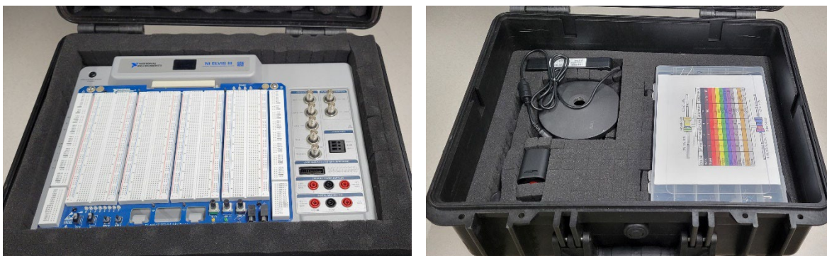
Figure 1: Portable lab equipment in travel case. Right: ELVIS-III in the first layer of case. Left: Second layer of case with document camera, cables, organizer with components, and test leads (under organizer).
