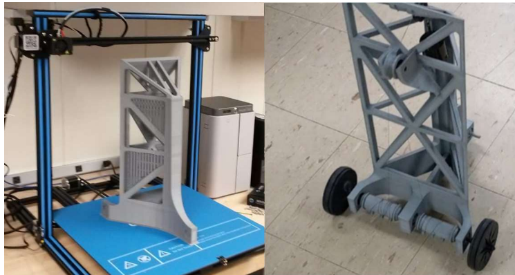
Figure 8 a. 3D printing the Ropebot components b. Completed assembly of the Ropebot
