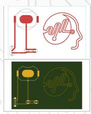
Students utilize Electronic Computer-Aided Design (CAD) to digitally refine and simulate their circuit designs before the milling process. This step enhances precision, troubleshooting skills, and overall mastery in microelectronics.
