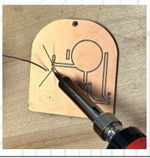
In the final step, students solder components onto their printed circuit boards (PCBs), bringing their digital designs to life and showcasing a wholistic understand of the electronics design process.
