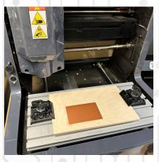
Using Computer Numerical Control (CNC), students manufacture printed circuit boards, bringing their digital designs to life with efficiency and precision. This step refines students' skills in translating digital designs into tangible, functional circuitry.
