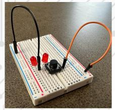
Students kickstart their circuit design journey by utilizing breadboards. Unlike traditional methods, breadboarding allows students to experiment and prototype circuits swiftly without the need for soldering.
