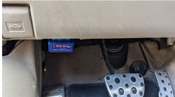
Figure 9: ELM327 Plugin Point near Drivers Feet [30]
